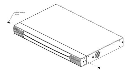
2. Use the screws you just removed, and the ones supplied with the rack mounting kit to screw the rack mounting brackets into both modules:
